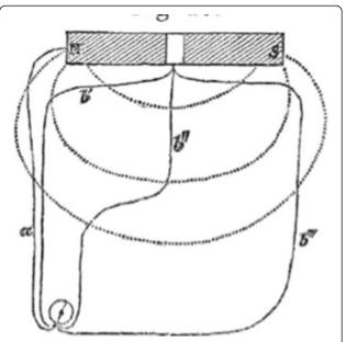
**Fig. 3** Picture of an experiment with different arrangements of wires (*a, b', b''*), magnet, and galvanometer. Note the lines of force drawn around the magnet. (Faraday 1852a, p. 34)
