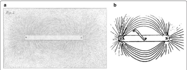
Fig. 2 a Iron filing pattern in case of bar magnet drawn by Faraday (Faraday 1852b, Plate IX, p. 158, Fig. 1), b Faraday's drawing of lines of magnetic force in case of cylinder magnet, where the experimental procedure, knife blade showing the direction of lines, is combined into drawing (Faraday, 1855, vol. 1, plate 1)
